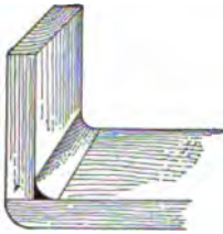
FIG. 173.—Use of Fillets in Pattern Making.
